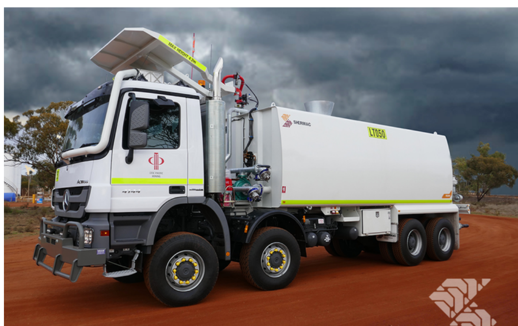
ON-ROAD WATER CARTS 18,000L water tank, to suit 8x4 chassis
